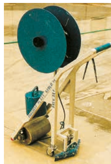
GROUT DRAGGER FOR MORE CONTROLLED LAYING
