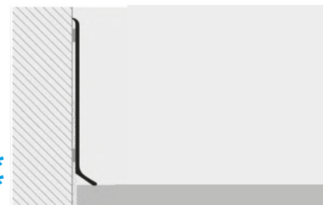
USE PROBAND FIX FOR FIXING THE PROFILE TO THE WALL
