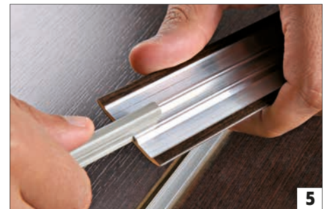
5) Keep the profile with the groove for insertion facing upwards and slot in the insert from the top downwards (if it does not slide easily, lubricate with water, silicone spray or vegetable oil).
