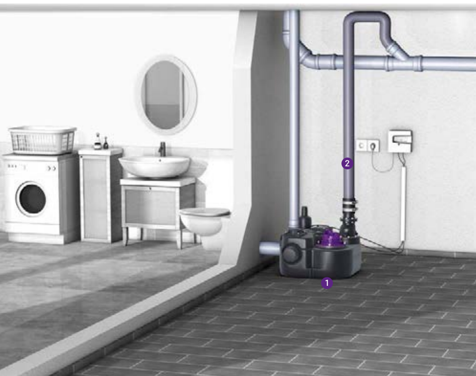
1 Lifting station 2 Pressure pipe
