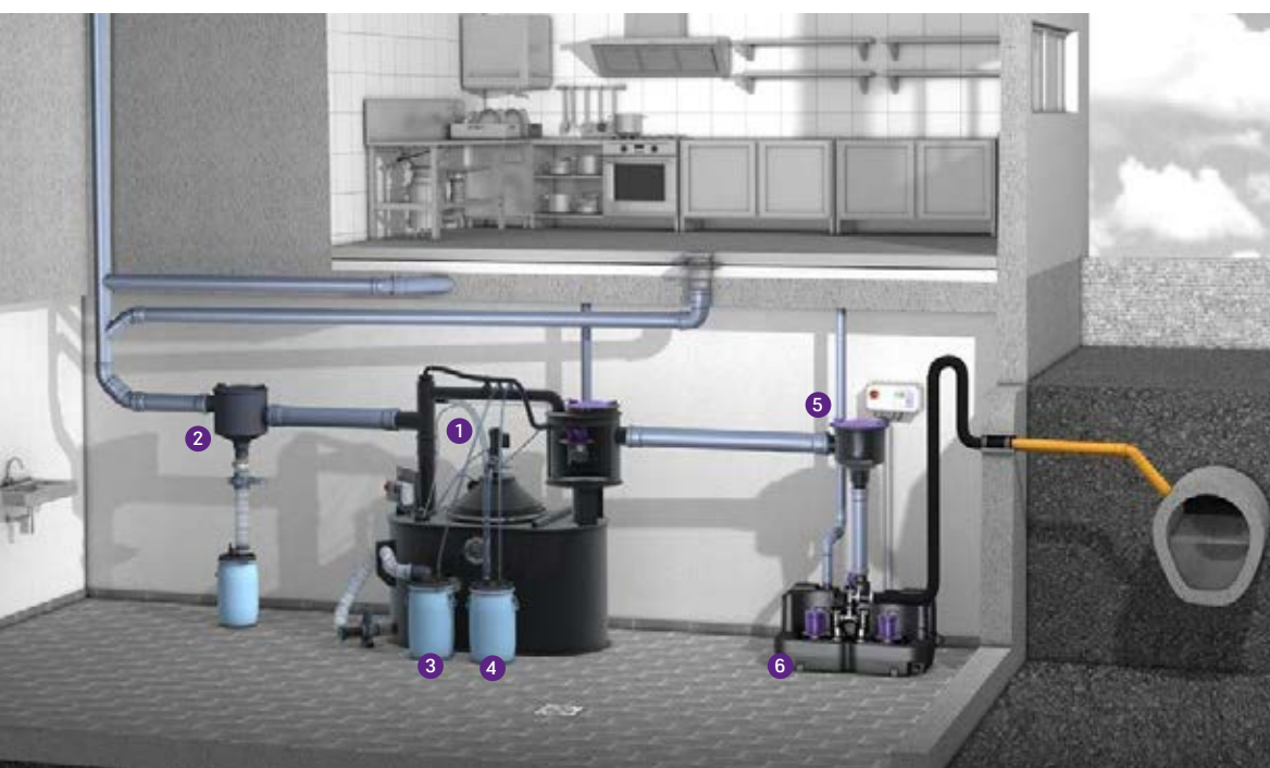
1 Grease separator 2 Pre-filter 3 Sludge storage tank 4 Grease storage tank 5 Sampling chamber 6 Lifting station
