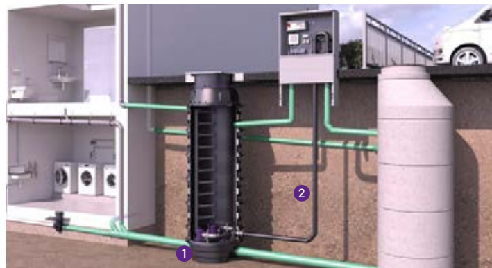
1 Hybrid lifting station 2 Pressure pipe
