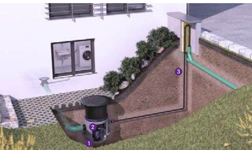
1 Pumping station 2 Pump 3 Pressure pipe
