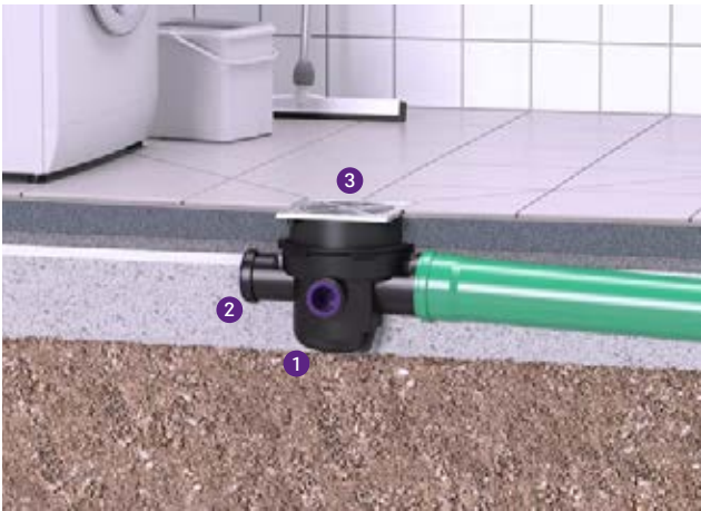
1 Drain 2 Inlet 3 Steel cover
