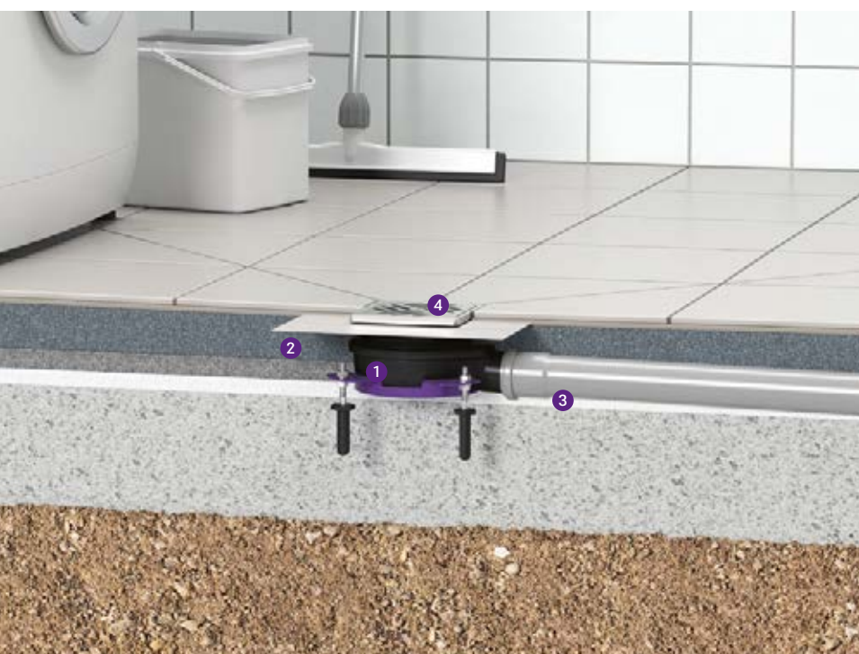
1 Drain 2 Waterproofing membrane 3 Drain pipe 4 Cover
