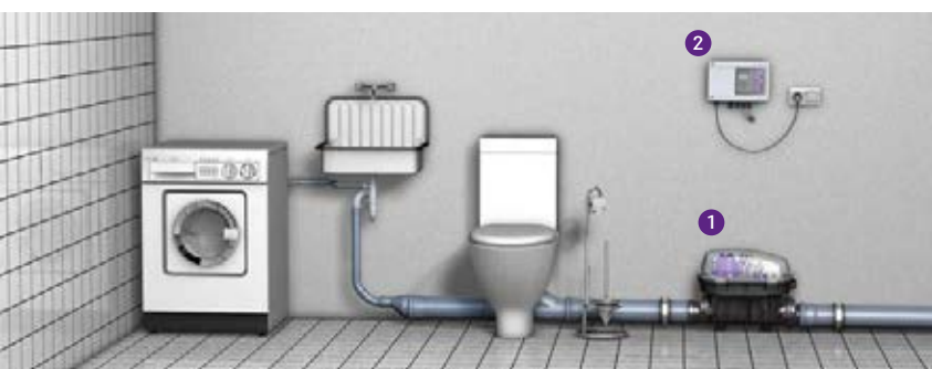
1 Backwater pumping station 2 Control unit
