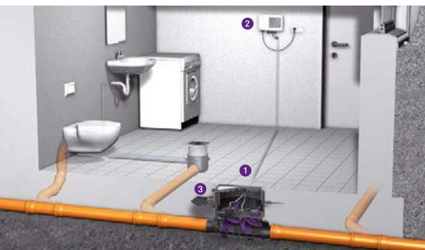
1 Backwater valve 2 Control unit 3 Sealing gasket set
